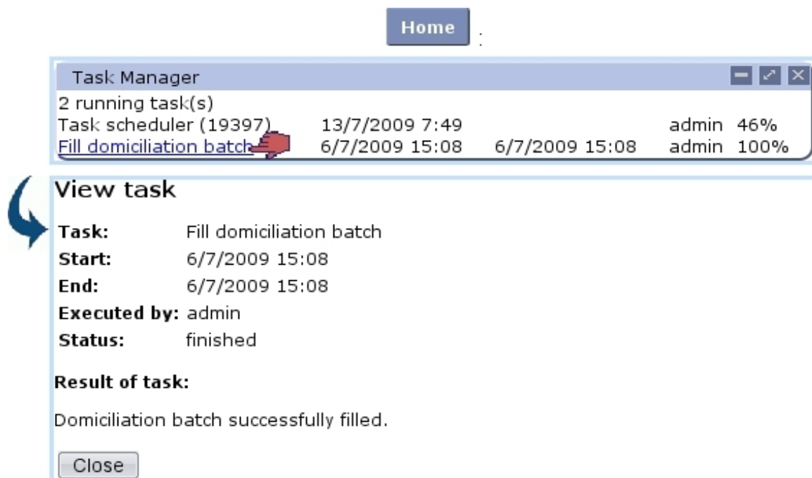
Figure 9.25: The system task manager event control, showing one running task and one finished ; accessing the details of the latter.
